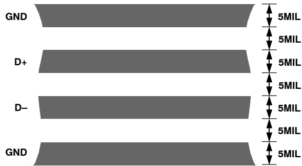
Figure 23. Typical Arrangement of Signal Tracks
